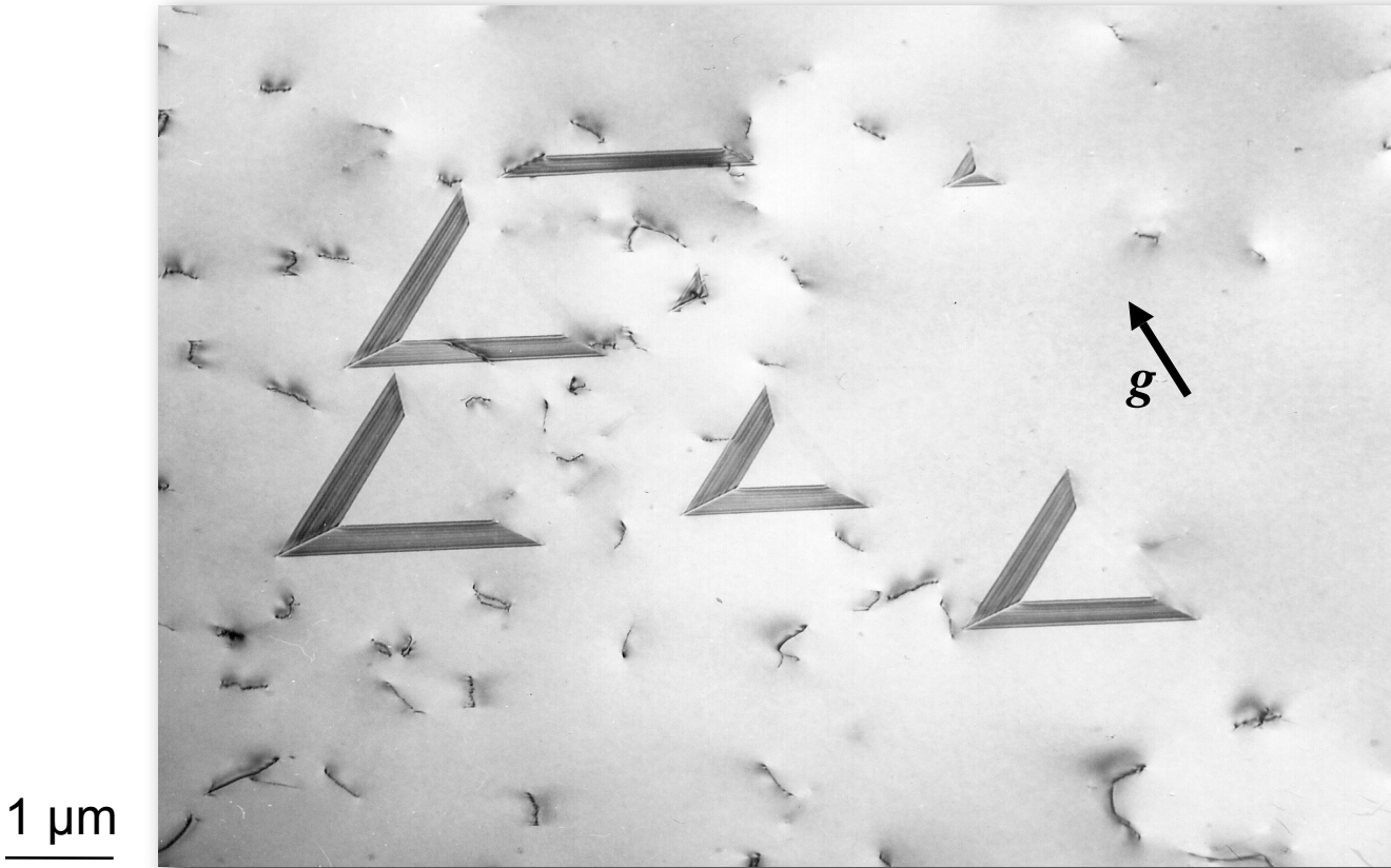
Stacking faults and threading dislocations in heteroepitaxial (111)CdTe/(001)GaAs. TEM bright field image, g diffraction vector.
