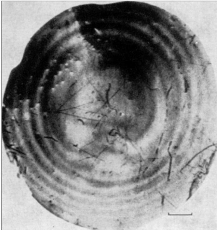
Striations in a Si wafer visualized by double-crystal X-ray topography.
